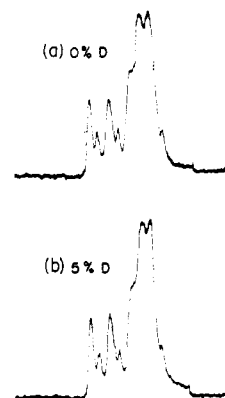
Fig. 1.—High resolution proton magnetic resonance spectra of pentaborane (a) normal isotopic content, (b) 5% deuterium.
